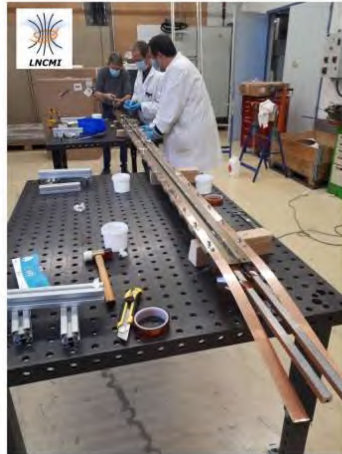
Insulated bus bars at the level of the connections & instrumentation wires in the magnet side on the left & in the cryogenic satellite in the right (14 Feb. 2022)
