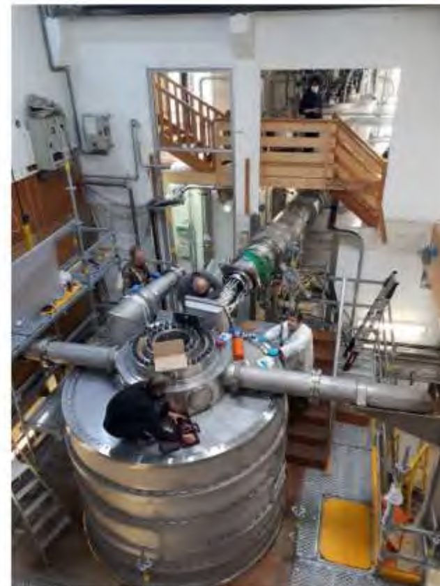
Mounting superinsulation layers on the magnet side (12 & 13 April)
