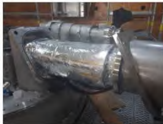
Welding of the cold mass of the cryogenic line to the magnet one
